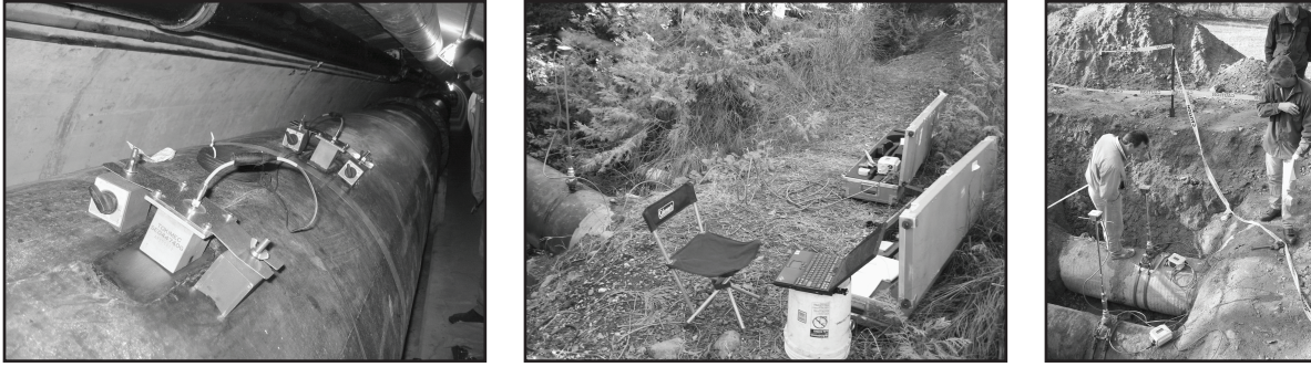
Figure D-2 Verification of system input volume through source meter tests (Courtesy of Water Systems Optimization)
