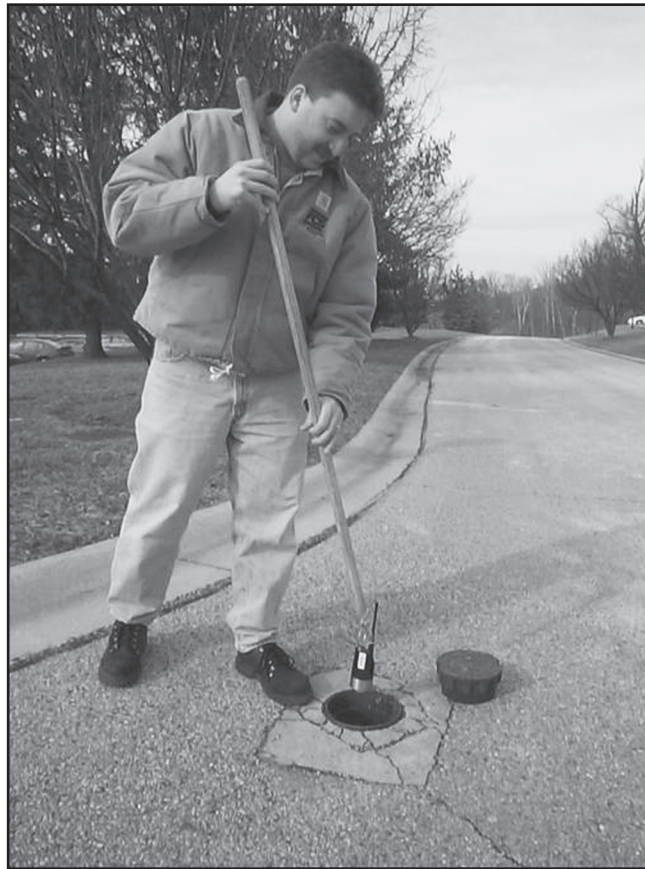
Figure 4-7 Leak noise loggers help to automate the leak survey process and provide consistent sounding capabilities for effective leak detection (Courtesy of Fluid Conservation Systems)
