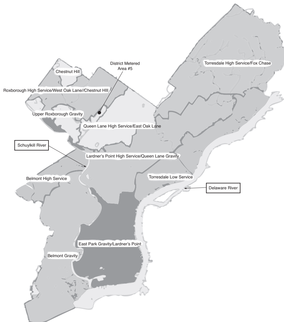
Figure 5-10 Pressure zones and DMA in the Philadelphia Water Department water service area (Courtesy of Philadelphia Water Department)
