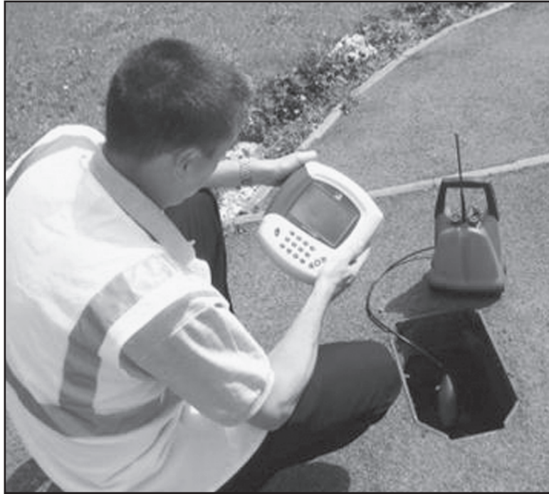
Figure 4-6 Leak correlators have become a standard pinpointing tool of the leak detection squad in many water utilities (Courtesy of Fluid Conservation Systems)
