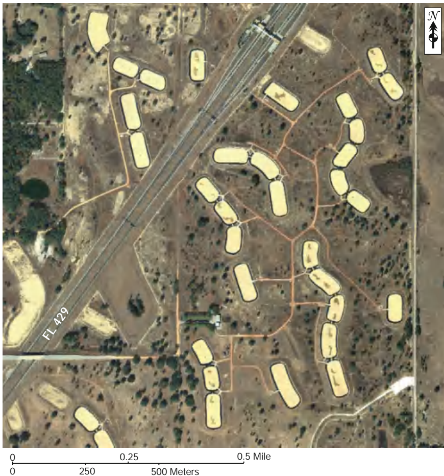
Fig. 15.8 Aerial photograph of part of Water Conserv II RIB Site 6A, western Orange County, Florida. Black border around the RIBs is the HDPE geomembrane liner on the side slopes (2011; Source USGS)
