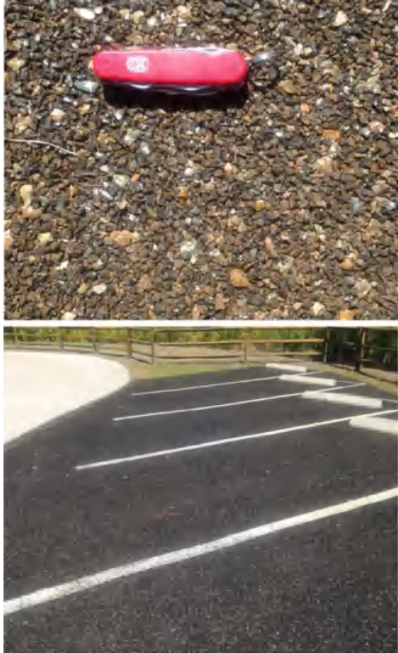
Fig. 23.7 Epoxy-bounded stone and rubber granules (KBI Flexi-Pave) used for a trail and parking lot, Wild Turkey Strand Preserve, Lee County, Florida
