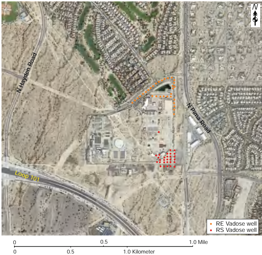
Fig. 17.5 Aerial photograph of the Scottsdale Water Campus (Arizona) showing locations of vadose wells
