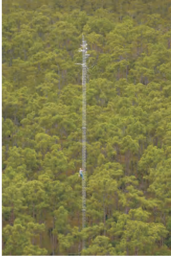
Fig. 4.4 USGS ET tower in the Big Cypress National Preserve. Note man on tower for scale. Source Shoemaker et al. 2011
