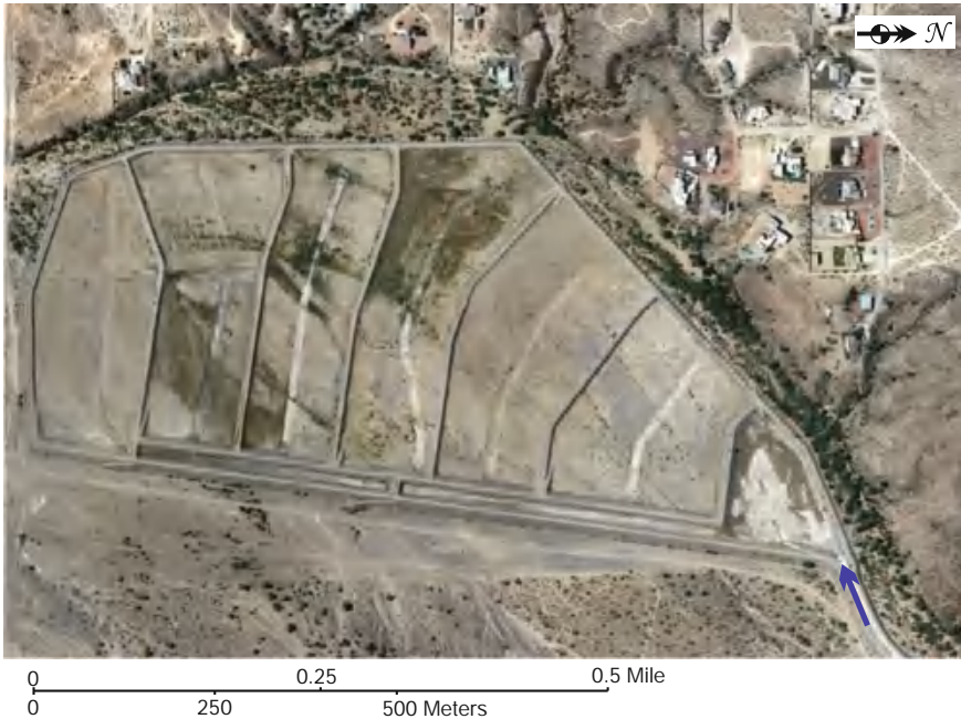
Fig. 15.11 Aerial photograph of the Agua Fria Recharge Project near Peoria, Arizona, in which the infiltration basin system is divided into cells (Source U.S. Geological Survey)
