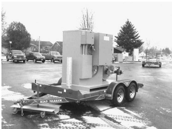
FIGURE 6-11. Small electric catalytic oxidizer. (Photograph provided by Catalytic Combustion Corporation.)
