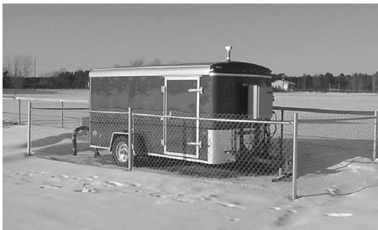
FIGURE 7-5. Trailer-mounted mobile soil vapor-extraction unit.
