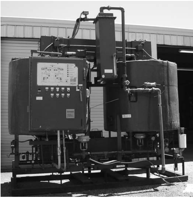
FIGURE 6-8. Regenerable granular activated carbon system. (Photograph provided by MK Environmental Inc.)
