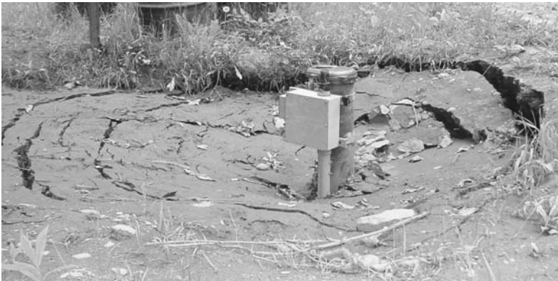
FIGURE 7-2. Sinkhole created by the mining of the formation by the extraction well.
