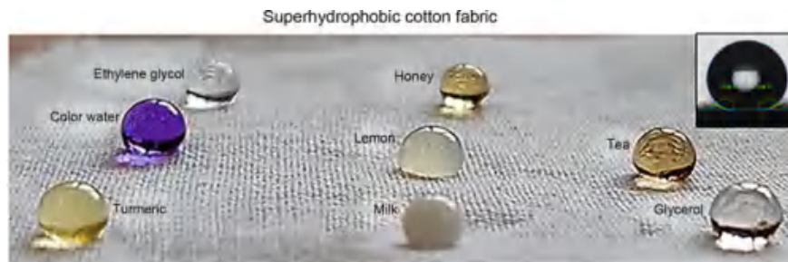
Fig. 9.11 Optical images of various droplets (color water, tea, milk, lemon, turmeric, honey, glycerol and ethylene glycol) on superhydrophobic cotton fabric. Liquid repellency for all liquid droplets is observed (adapted from Chauhan et al. 2019)
