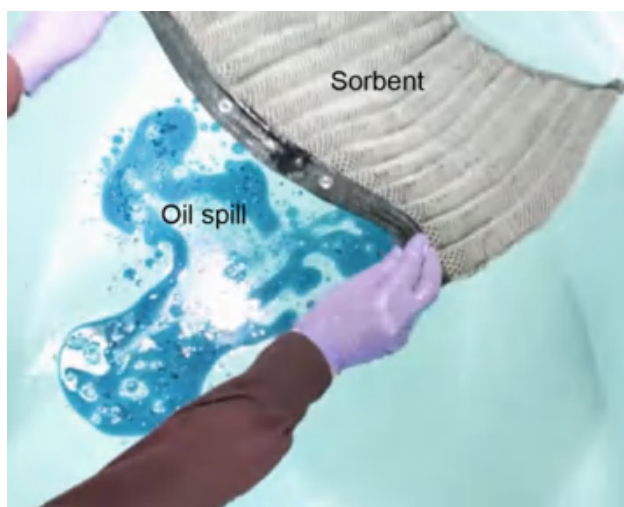
Fig. 9.A.2 Photograph of the sorbent sucking up oil spill (adapted from Bhushan 2018)
