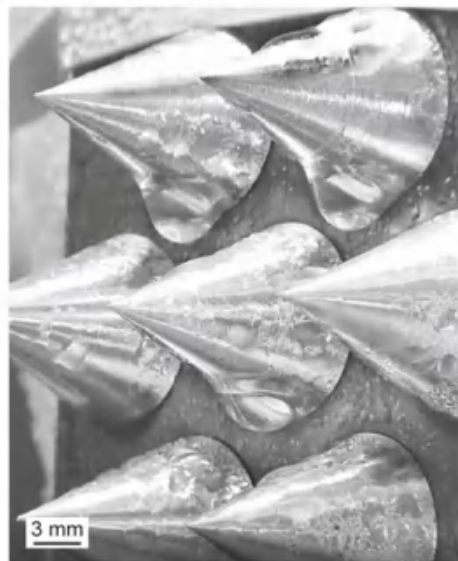
Droplets falling from the top cone coalesce with droplets stuck to cone underneath and get collected fast
