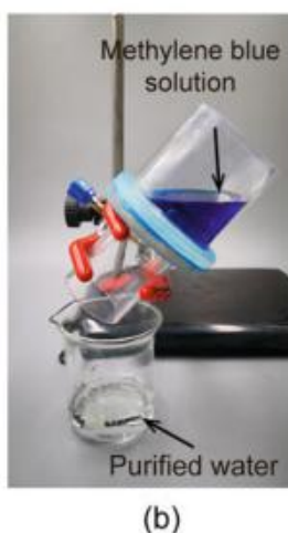
Fig. 9.28 Schematic of water purification process showing purification of methylene blue aqueous solution on superhydrophobic/superoleophobic stainless steel mesh. a Photocatalytic degradation of contaminants occurs by UV irradiation. Pure water passes through the mesh. The mesh could be reused after heating it up. b The methylene blue in water was degraded during UV irradiation and transparent purified water flowed down into a beaker (adapted from Li et al. 2019b)
