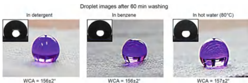
Fig. 9.12 Optical images of water droplets on treated cotton fabric after 60 min washing in detergent solution, benzene and hot water (80 °C) via ultra-sonication method, showing its excellent washing ability. Inserts are contact angle images. Water contact angles are also presented (adapted from Chauhan et al. 2019)
