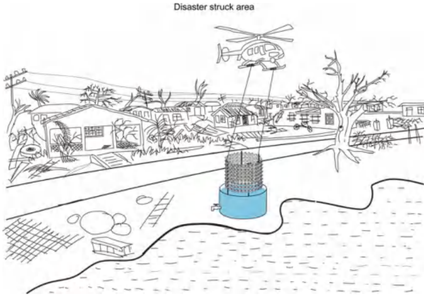
Fig. 6.2 Schematic of a portable water harvesting tower being dropped by a helicopter in an emergency zone on an island (adapted from Bhushan 2020)
